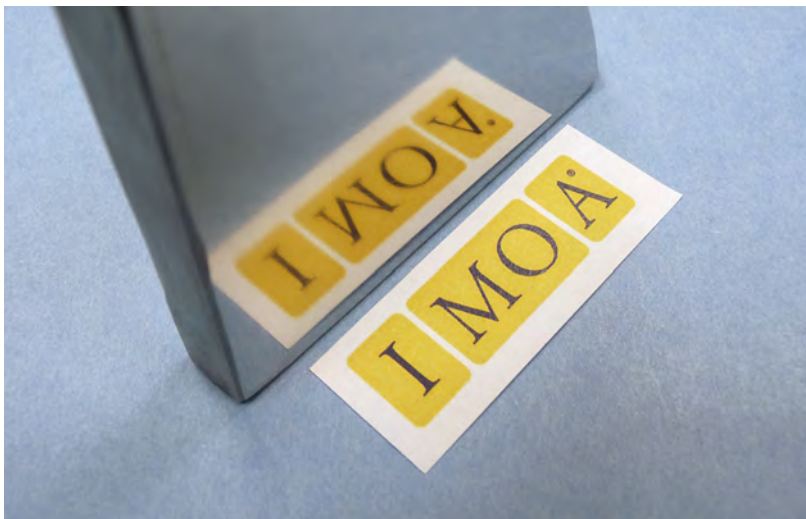
Figure 7. Electropolished 2205 plate (Sample provided by DCI, Inc.)
