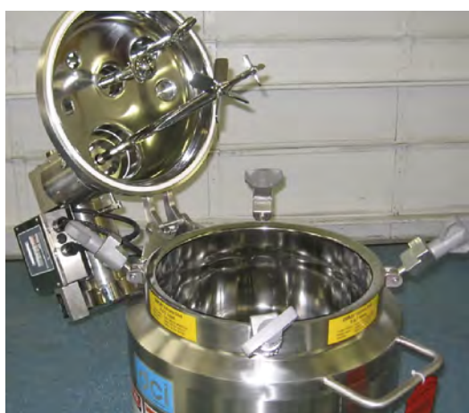
Figure 1. Pharmaceutical R&D vessel fabricated from 10 gauge 2205 duplex stainless steel sheet and 3/16 inch (4.8 mm) thick 2205 plate. Product contact surfaces were electropolished to an ASME BPE – SF4 finish. (Courtesy of Genentech)
