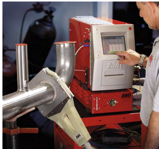
Figure 6. Automatic orbital welding of stainless steel tubing (Courtesy of Arc Machines, Inc.)
